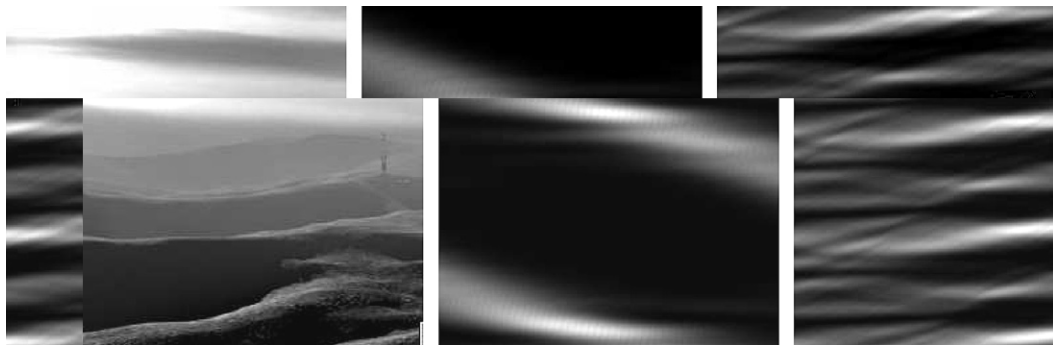
Fig. 10. A photographic image (of dimensions 256 \times 256 ) “reconstructed” with wave lengths of 10 and 5 pixels, respectively, using an equidistant setup of N = 101 beams.
